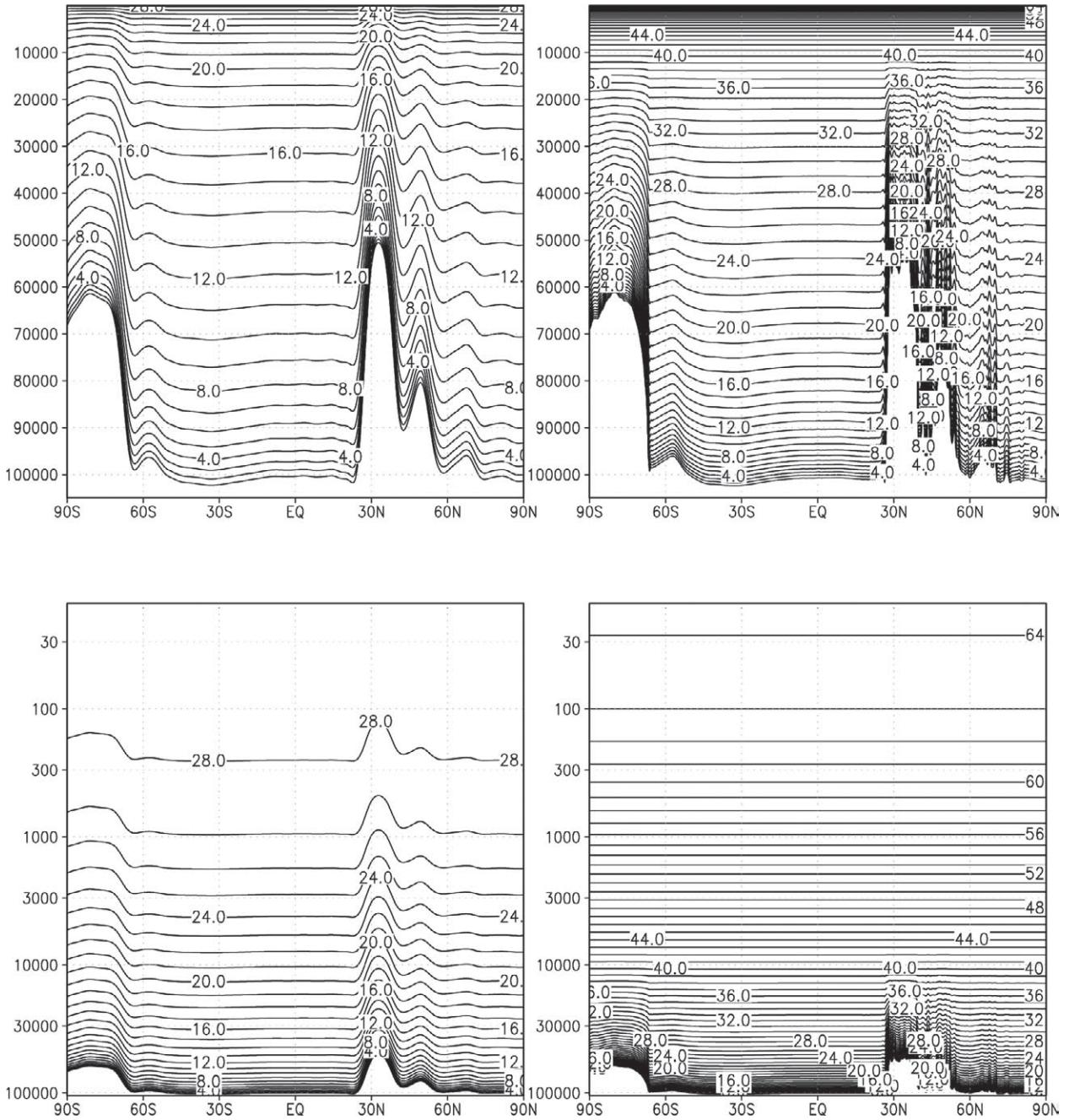
**FIG. 10.** The vertical structure of model levels as a meridional cross section at 90°E. (left) RI (28 sigma layers) and (right) CFSR (64 sigma–pressure hybrid layers). (top) A linear function of pressure to emphasize resolution in the troposphere; (bottom) log(pressure) is plotted to emphasize stratosphere.
