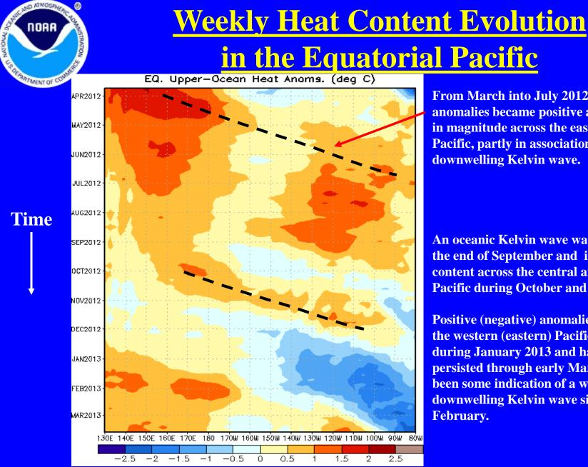
From March into July 2012, heat content anomalies became positive and increased in magnitude across the eastern equatorial Pacific, partly in association with a downwelling Kelvin wave.
