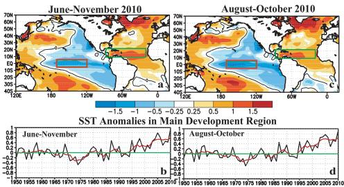
Fig. 6. (Top) SST anomalies (°C) during (a) Jun-Nov 2010 and (c) Aug-Oct 2010. (Bottom) Time series of consecutive area-averaged SST anomalies in the MDR during (b) Jun-Nov, and (d) Aug-Oct. Red line shows the corresponding 5-yr running mean. Green boxes in (a, c) denote the MDR. Anomalies are departures from the ERSST-V3b (Smith et al. 2008) 1971-2000 period monthly means.
